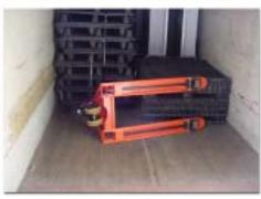
The "old way" meant that the driver had to man handle the pallet truck to tip it on its side.
