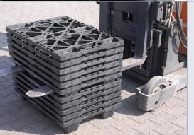
Pallet stack is accessible with forklift tine.
